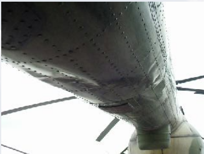
Typical wrinkling in the tailboom region
